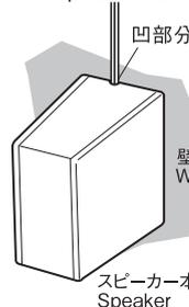
②Lead the speaker wire through the exit section for speaker cable on the upper side of enclosure and fit the speaker on the wall according to "Installation 4". (See to Fig. 6/8)
